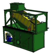
direction of flow. The deck is approximately 6.7m<sup>2</sup> being 1.4 m wide by 4.8 metres long. Separated solids are discharged off the front of the shaker outside the end face of the pump tank. The shaker is powered by 2 No. 6.2kW electric motors fitted with eccentric weights. The motors have Direct-On-Line starting.
