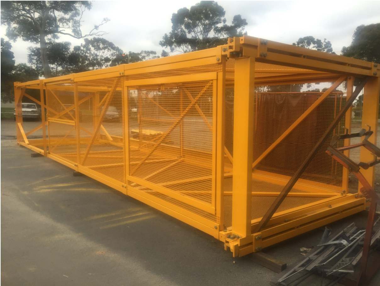
Hoist Frame delivered as Pre-Assembled. Monorail and Hoist to be assembled on site.
