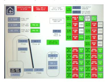
Each kettle is fitted with a total of 10 heating elements, totaling 175 kW of heating.
