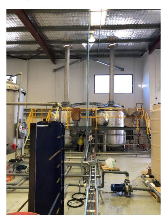
The plant consists of two 4000 litre kettles, fitted with 5M distilling towers. The plant can process upt to 3500 litres of mash per batch run, extracting up to 400 litres of Ethanol, at an input alcohol level of 17%. Assuming a batch time of 4 hrs per kettle, operating for 24 hrs per day, 7 days per week, the theoretical production capacity is 1.35-1.5M litres per annum.
