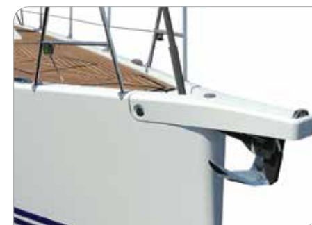
Optional white painted carbon bowsprit with integrated anchor fitting
