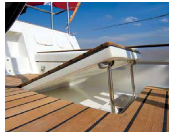
Top: Adjustable folding foot chocks
