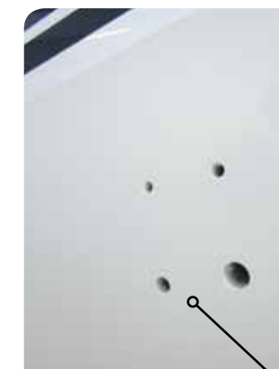
Recessed through-hull fittings
