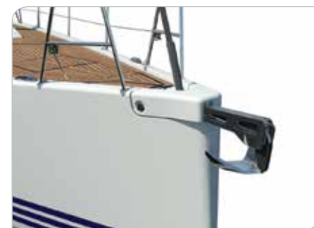
Standard GRP cowl with integrated anchor fitting
