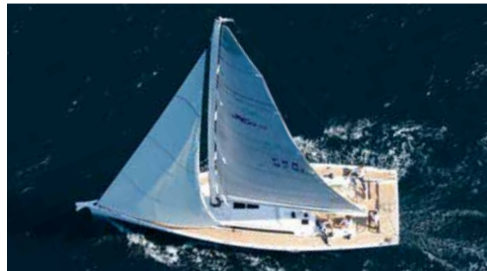
Left and centre: A custom-designed three-spreader alloy rig is supplied as standard, with a higher aspect carbon mast and boom available as an option
