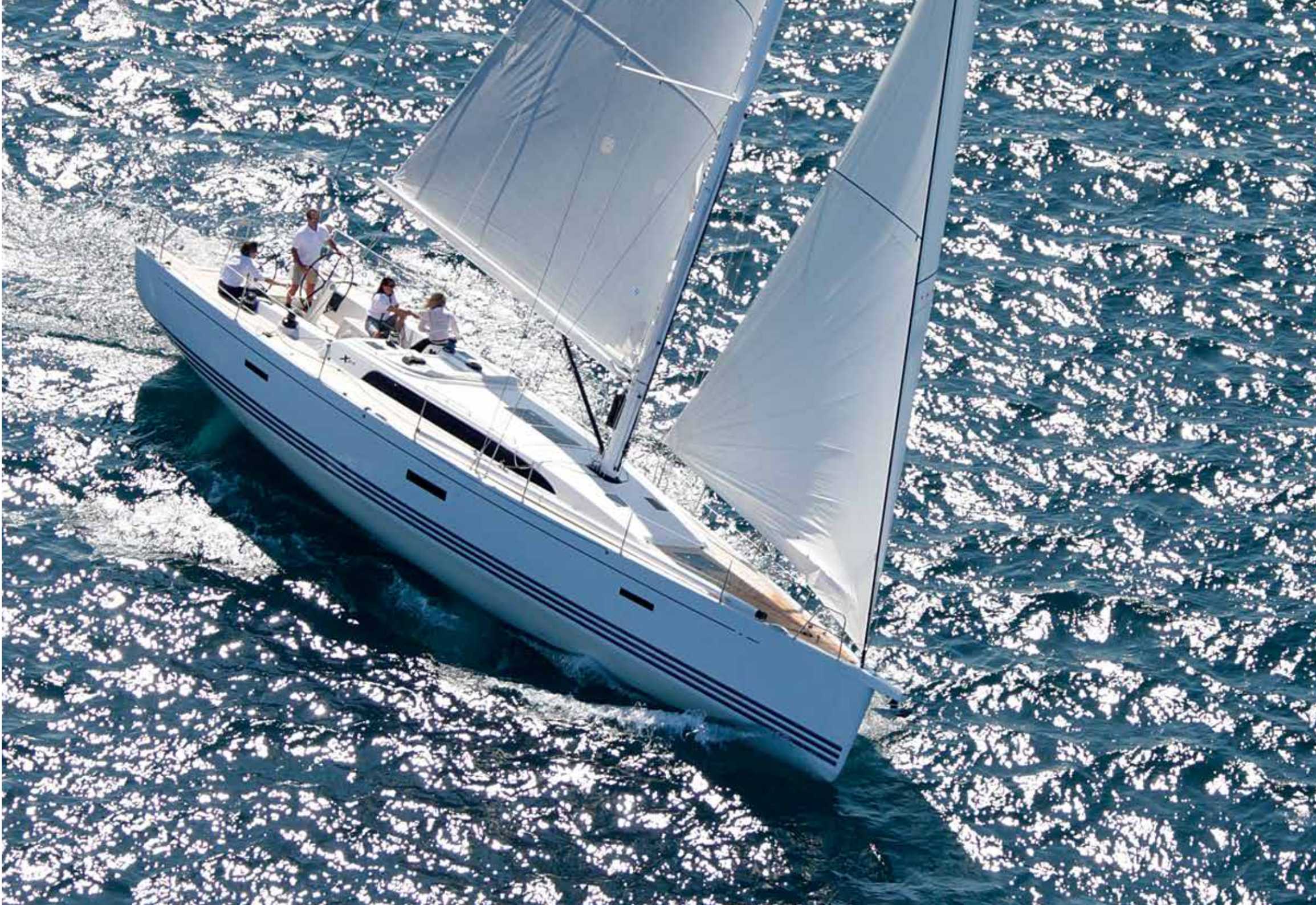
Left and centre: A custom-designed three-spreader alloy rig is supplied as standard, with a higher aspect carbon mast and boom available as an option
