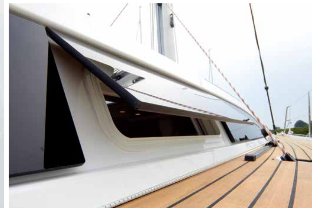
Opening portlight windows and recessed deck fittings
