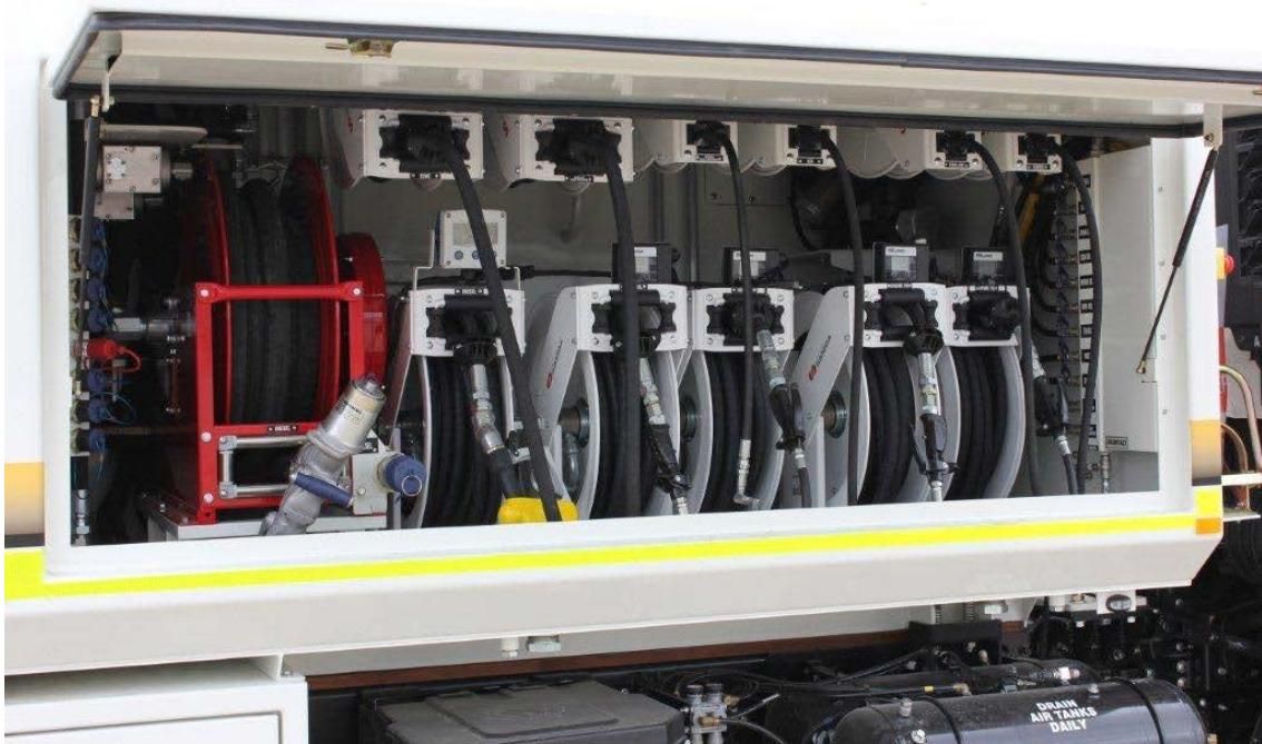
Uncoil the hose reel to desired length. It can be locked by means of the latch mechanism which is a clicking noise heard after each half resolution of the drum. By gently pulling the hose until the clicking noise has stopped, the latch is released and the hose is automatically recoiled.
