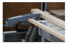
Beam turning device
