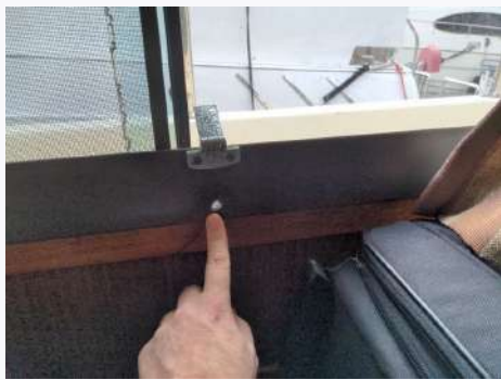
Ref # 7.7 - Corrosion hole in port side window bezel.
