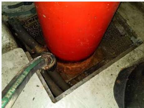
Ref # 19.3 - Gen Set bay cylinder. (Corroded)
