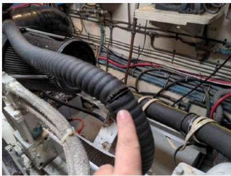
Ref # 8.12 - Air hose return hose split on port engine,
