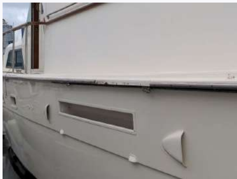
Ref # 3.2 - Section of gunnel strip missing
